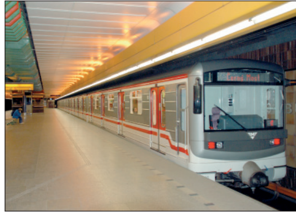
A retrofitted 81-71M train at the Nové Butovice station
